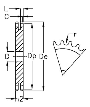
C = 4 D = 30 De = 480.4 Dp = 465.26 For chain size = 1 1/4 x 3/4 For chain type = 20 B-2 h2 = 54.6 L = 18.2
